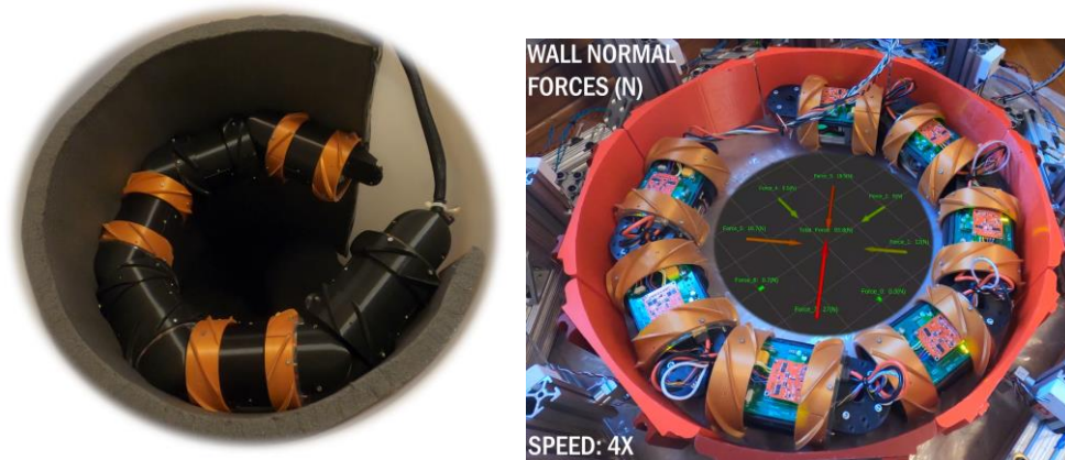
Figure 7: Left image: EELS Prototype for Force Compliance Testing demonstrating vertical traversal in a barrel. Right image: load leveling validation.
