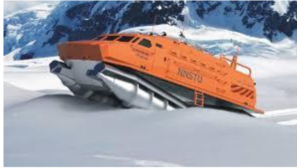
Figure 3: Universal arctic rescue vehicle (URV) (Image M.Y. Sandakov Et. Al)
